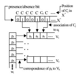
Fig. 1. Data structure showing parameters relationship in the family  $f_i = (x_i^*, w_i)$ .
